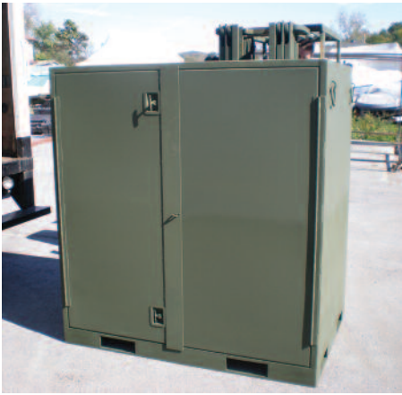
The US Marine Corps uses powder-coated boxes to service air-conditioning units in the field. Extreme Powder Coating coats the boxes with a government-approved primer before it sprays on a green liquid top coat.
