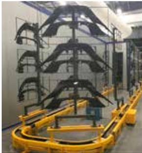
Cart provides a full 30-minute dwell time in paint booths or ovens. Cart can be equipped with automatic rotation to meet system requirements, allowing the design of a more efficiency, smaller finishing system with lowered utility costs.
